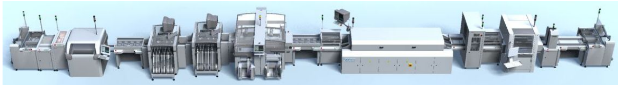
Figure 1 Manufacturing line for surface mounted technology
