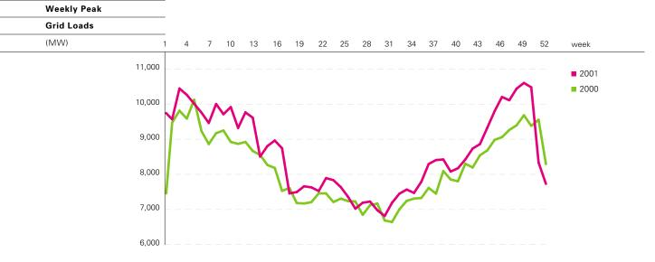
The maximum load on the Czech Republic Power System in 2001 was 10,604 MW measured on Thursday, December 13 at 14:00. This is 476 MW higher than the highest load measured in 2000.
